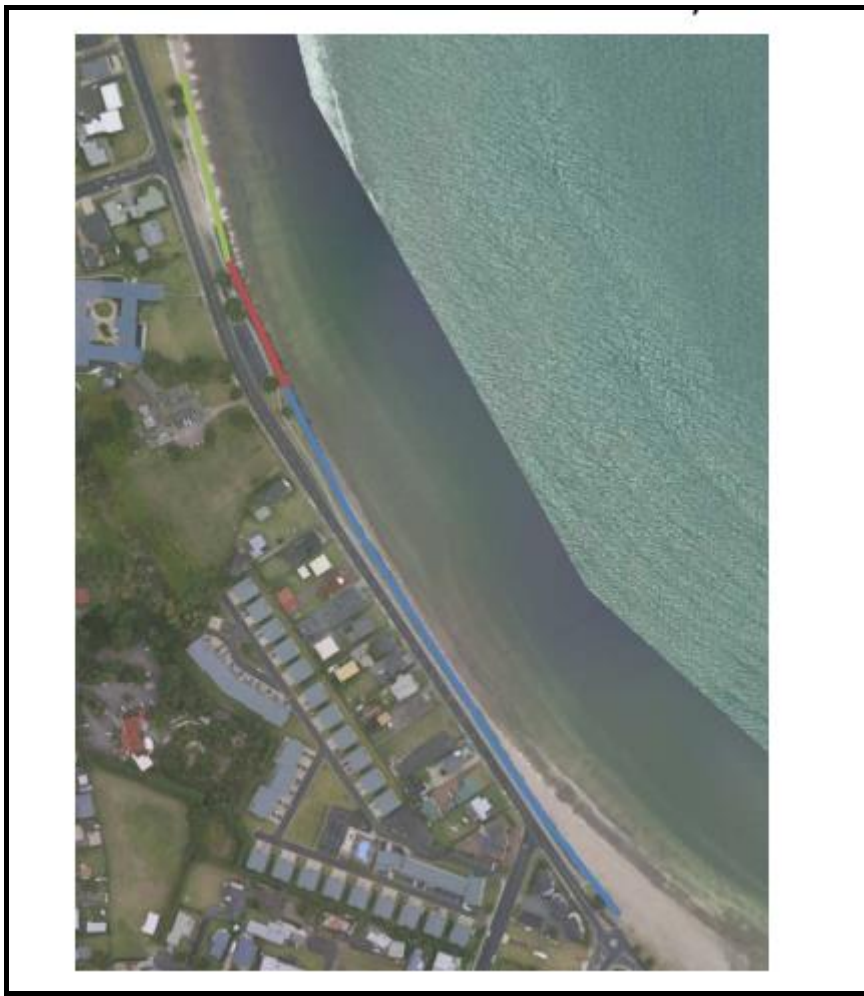
Figure 1 – Aerial photograph displaying existing seawalls at Buffalo Beach (blue line – NZTA seawall, red line – toilet block, green line – extension wall to the toilet block)
